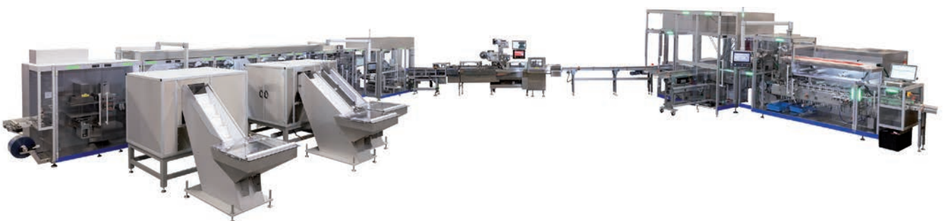
Packaging line for tubes and applicators with pick & place units
