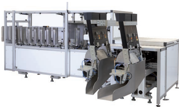
Packaging line for tubes and applicators with pick & place units
