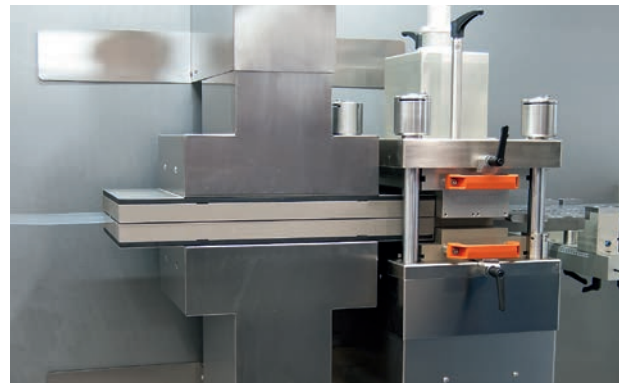
Thermo- / coldforming station
